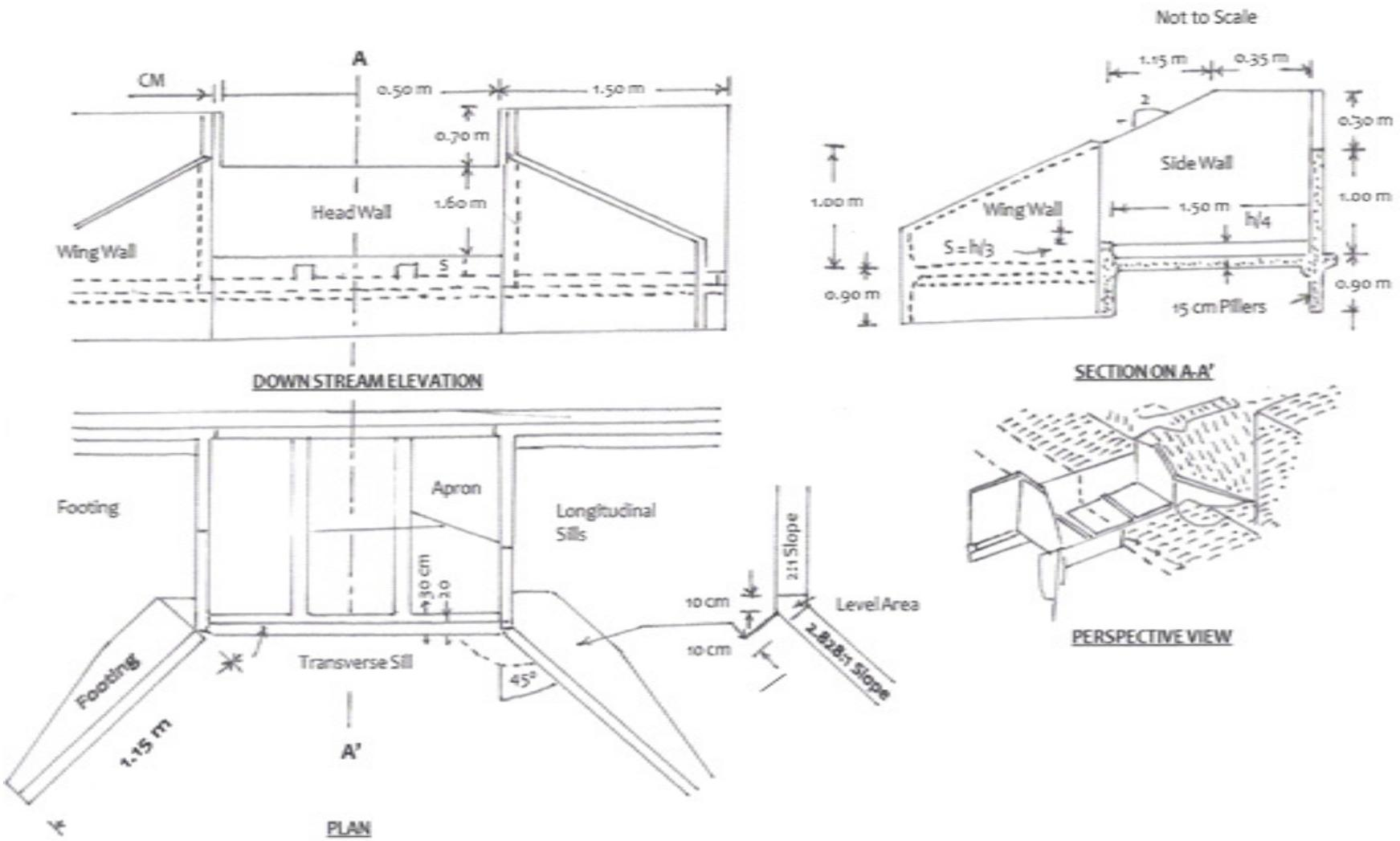
Design of Drop Spillway to be constructed at a place in a gully having width of 1.0 m and catchment area 1.00 and net drop 0.50 m Taking rainfall intensity for duration equal to time of concentration of watershed and design return period of 25 years , as 120 mm/hr . The coefficient of runoff for the watershed is 0.3.
